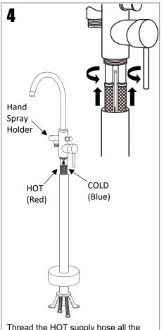
Thread the HOT supply hose all the way into the threaded hole in the bottom of the faucet body nearest the hand spray holder, and the COLD supply hose in the far hole. The connections on the Faucet Body are also marked H and C. Hand tighten or apply light torque with pliers. No need to overtighten.
