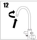
Re-install the aerator at the end of the spout. Be sure the black rubber washer is in place. Hand-tighten firmly.
