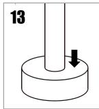
Slide the Floor Escutcheon (4) down to the floor and seal with silicone caulk.
